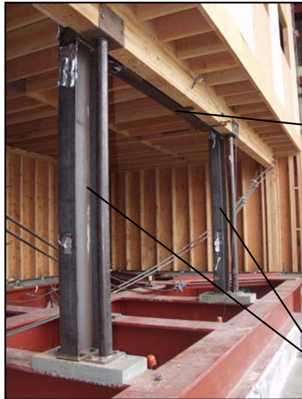
View of Full-Scale Apartment Building Model Prior to Installation of Stucco on Exterior and Gypsum Board on Interior
