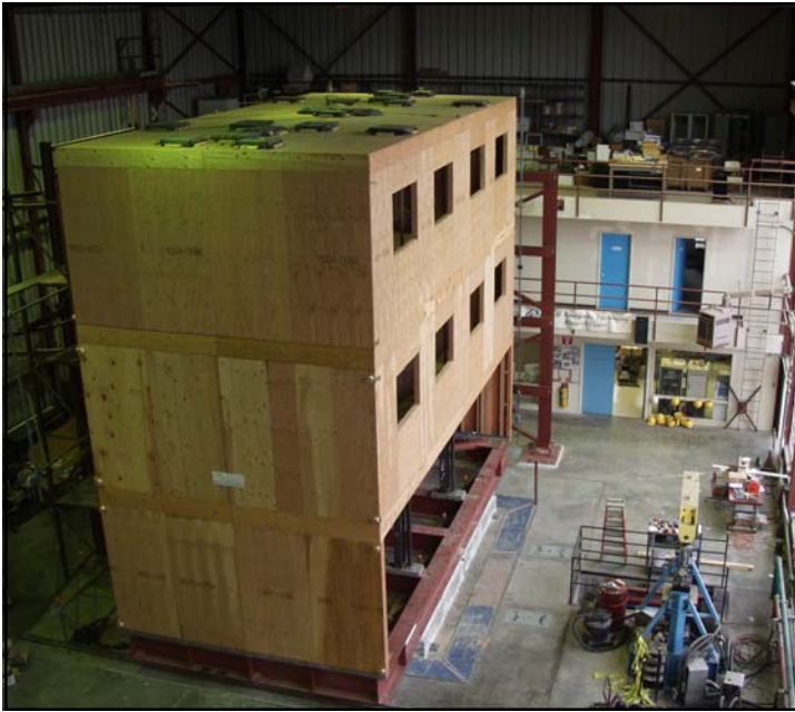
View of Full-Scale Apartment Building Model Prior to Installation of Stucco on Exterior and Gypsum Board on Interior
